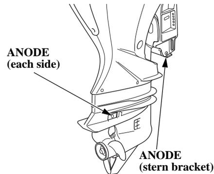
The anode is a sacrificial material which helps to protect the outboard motor from corrosion.
