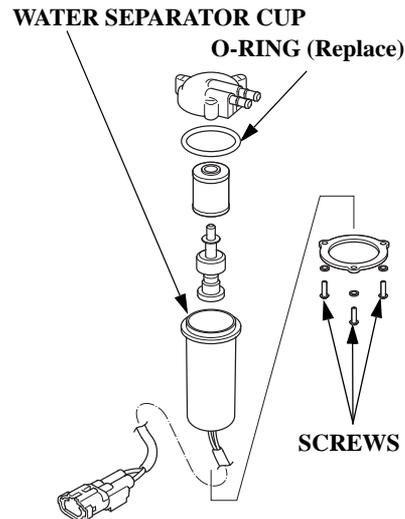
5. Remove the three screws holding the fuel filter with water separator, delete the water or deposit from the inside of the cup.
