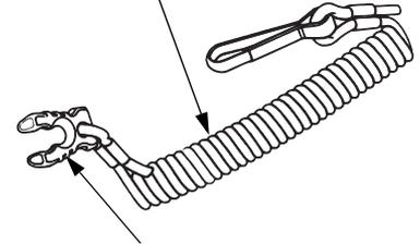
The emergency stop switch clip must be engaged with the emergency stop switch or the engine will not start. When the emergency stop switch clip becomes disengaged with the emergency stop switch the engine will stop immediately.
