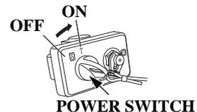
3. Insert the key to the power switch and turn it to the ON position.
