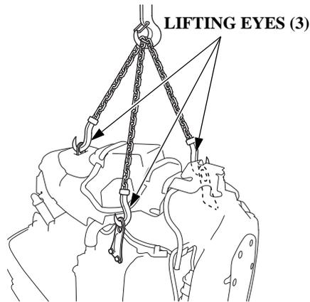
Before installing the outboard motor on the boat, hang the outboard motor with the hoist or equivalent device by attaching the three lifting eyes to the outboard. Use the hoist which allowable load is 300 kg (661 lbs) or above.
