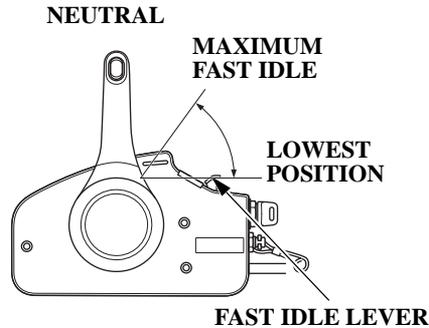
The fast idle lever will not move unless the remote control lever is in the NEUTRAL position. Conversely, the remote control lever will not move unless the fast idle lever is in the lowest position.
