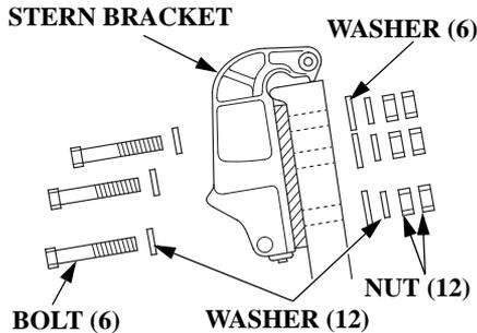
1. Apply the silicone sealant (Three Bond 1216 or equivalent) to the outboard motor mounting holes.
