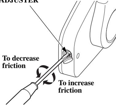
Check whether the remote control lever moves smoothly. Friction of the lever can be adjusted by turning the control lever friction screw right or left.
