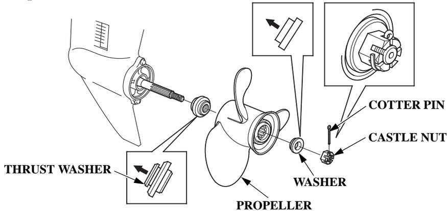
If the propeller is damaged by striking a rock, or other obstacle, replace the propeller as follows.
