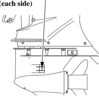
The engine cooling water is drawn into the engine through this port.
