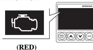
The PGM-FI indicator turns on and the buzzer sounds when the engine control system is faulty.
