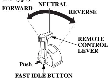
Use the fast idle button and the remote control lever to adjust the engine speed without gearshift when warming up the engine.
