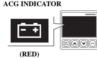
The ACG indicator turns on and the buzzer sounds when the charging system is faulty.
