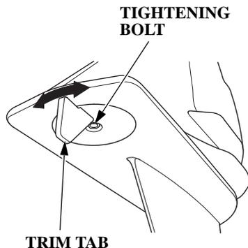
If the steering wheel/handle is pulled to the side while running at full speed, adjust the trim tab so that the boat runs straight ahead.
