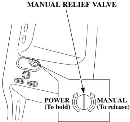
After tilting the outboard motor, turn the manual relief valve clockwise securely. The manual relief valve must be tightened securely before operating the outboard motor or the outboard motor could tilt up when operating in reverse.
