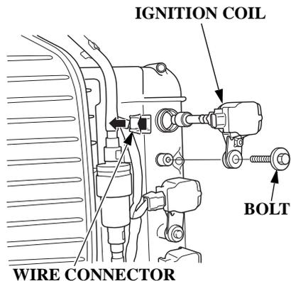
3. Disconnect the wire connector from the ignition coil by pushing on the lock tab and pulling on the connector. Pull on the plastic connector, not the wires.
