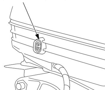
The power tilt switch located on the outboard motor pan is a convenience switch for tilting the outboard motor for trailering, or performing outboard maintenance. This power tilt switch should only be operated with the boat being stopped and engine off.
