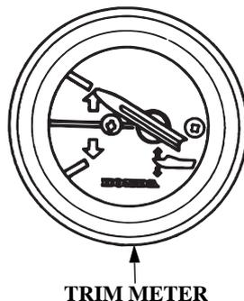
The trim meter has a range of -4° to 16° and indicates the trim angle of the outboard motor. Refer to the trim meter when using the power trim/tilt switch to achieve proper boat performance.
