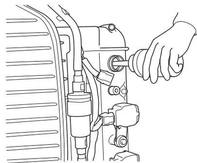
4. Put a teaspoon of engine oil into each spark plug hole to lubricate the inside of the cylinders. Reinstall the spark plugs.
