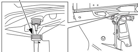
4. Remove the flush plug connector from the outboard motor.
