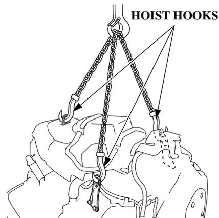
2. Set the hoist hooks against the lifting eyes and hang the outboard motor to remove it from the boat.
