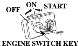
3. Turn the engine switch key to the START position and hold it there until the engine starts.
