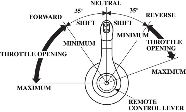
Shifting gear into forward, reverse, or neutral and the engine speed adjustment can be performed with the remote control lever. It is necessary to pull up the neutral release lever to operate the remote control lever.
